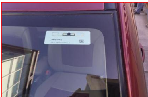
Factory fitted RFID/Fastag ( Front Windshield)
