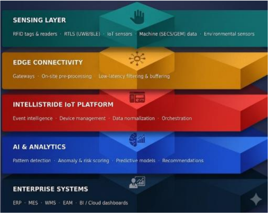
Figure 3 — IntelliStride Technology Architecture for Semiconductor Operations
